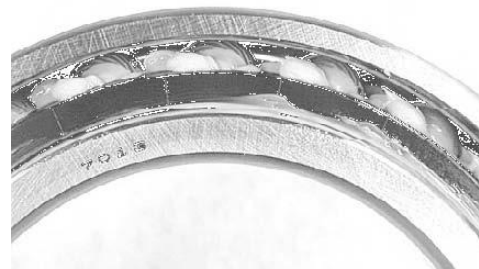
Fig. 1.23 Grease Packed Cylindrical Roller Bearing
