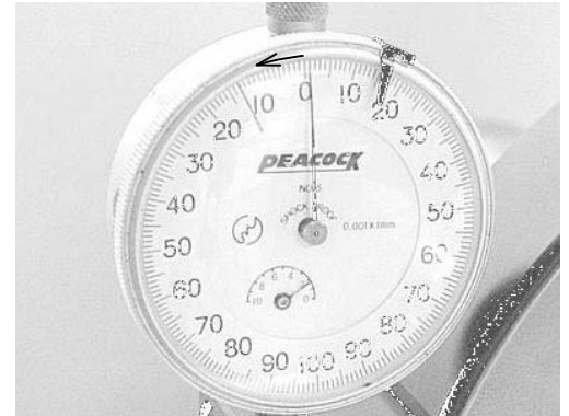
Fig. 1.11 Setting the GN Gauge
